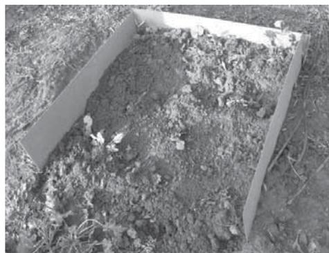
Image 2 Pair of microplot for the collection of runoff and sediment.
